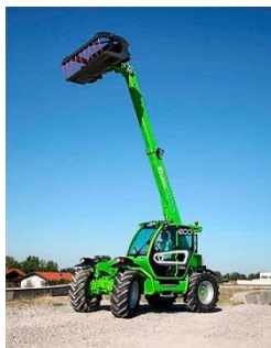
Figure 4: Tehelendler with hybrid drive - Turbofarmer 40.7 Hybrid-Merlo
